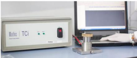
**Analysis of thermal conductivity**, specific heat, thermal diffusivity and effusivity of any type of solid, liquid, paste and powder material.
