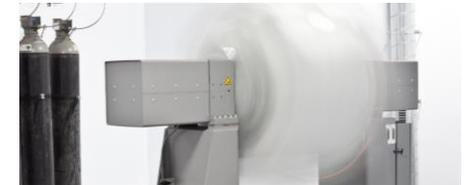
**Characterisation and modelling of sensors and inertial measurement units**. Platform testing (Hardware in the Loop). Acutronic 2-axis motion simulator with detachable thermal camera.
