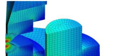
**Structural analysis of components** through simulation by the finite element method: stresses and deformations for static and dynamic loads.
