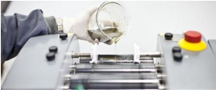
**NPs dispersion processes**. High shear force technology (three roll mill, ultrasonic homogeniser).
