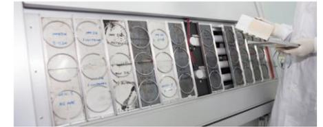
**Accelerated environmental ageing**: UV radiation, water and temperature, according to standards. Salt fog chamber (UNE-EN ISO 9227), QUV (UNE-EN ISO 11507, UNE-EN ISO 4892-3). Alternating immersion test. For other standards, please enquire. Thermal/humidity tests.
