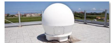
**Development and characterisation of navigation systems** (multi-antenna GNSS, multi-receiver), data fusion from other sensors (INS, odometry, etc.). **Experimental installation** composed by a radome and high precision 2-axis rotary table.
