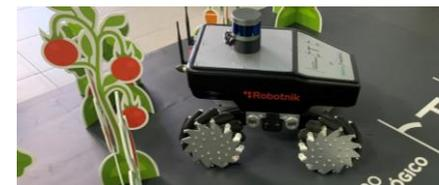
**Guidance, navigation and control of autonomous unmanned vehicles**. Test robot with differential and holonomic movement, 3D LIDAR sensors with 360° vision.
