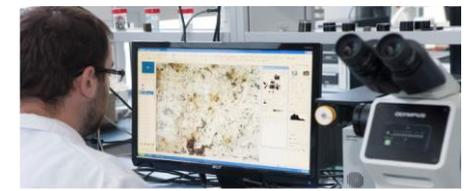
**Metallographic and microstructural analysis**, grain size, porosity, phases, cracking. Surface analysis of coatings. Thickness determination. Microscopic analysis (OM).
