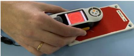
**Spectrocolorimetry**. Comparative-quantitative analysis of colour in materials and products.
