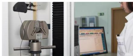
**Mechanical characterisation of polymeric materials** (plastics, thermosets and elastomers) and metals. Tensile, bending and compression tests.
