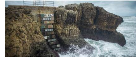
**Degradation tests against the environment** under real operating conditions (corrosion, biofouling) Marine laboratory in the open sea, MCTS El Bocal.
