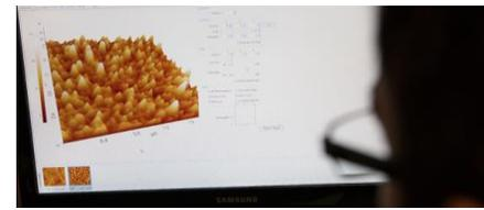
**Analysis by atomic force microscopy (AFM)**. Morphological analysis of nanomaterials. Imaging, topography, electrical, magnetic, thermal and mechanical properties.
