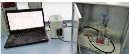
**Electrochemical tests**. Metals and metallic coatings, (potential and corrosion rate, polarization resistance, etc.); organic coatings (EIS, impedance, ACET tests according to UNE-EN ISO 17463).
